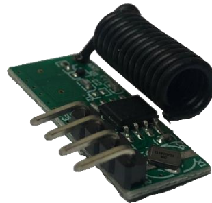
Figure 15: RF Receiver, RF Receiver Input and correctly installed state.
