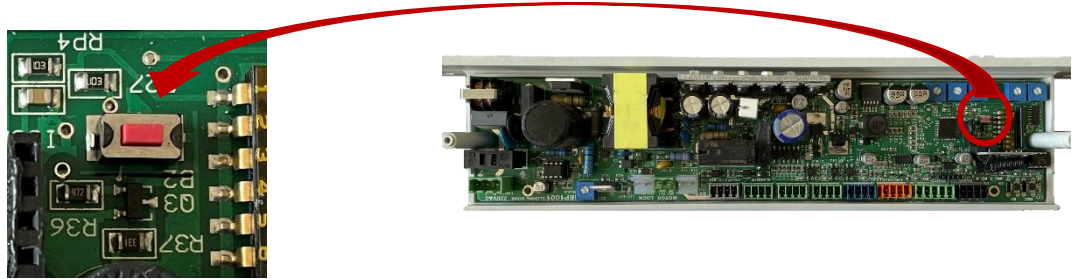
Figure 20: The position and close-up view of the Reset Button on the card.
